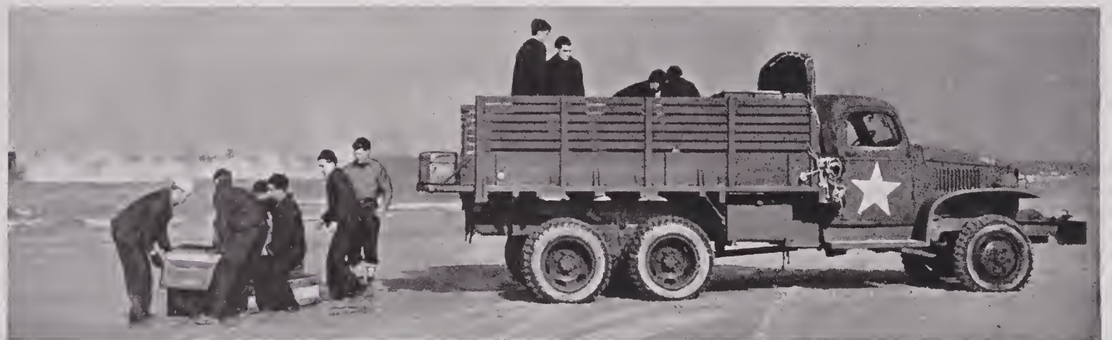
FIGURE 100. Last stage in LCV cargo-landing routine. Men lift cargo on to standard land truck. (In Fort Story demonstration, LCVs landed only about 30 tons in 90 minutes.)
